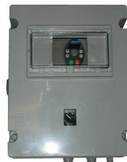
Electrical control panel with speed controller
