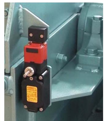
safety switch on hatch opening
