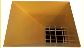
Concentrated minerals and additives hopper on mixer cover with sliding flap
