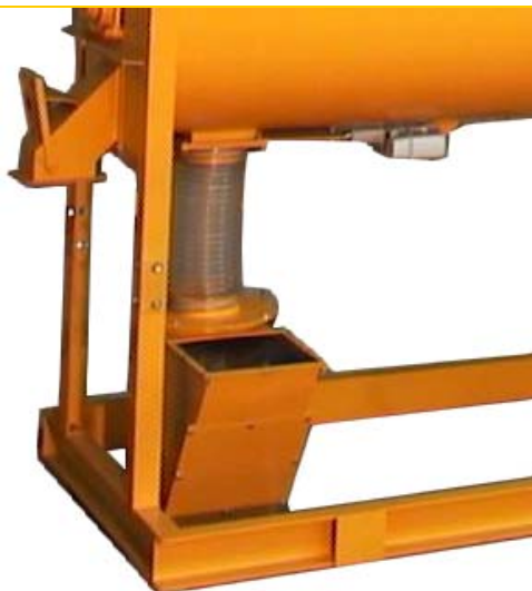
Inlet for auger downfeed
