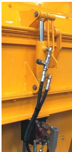
Hydraulic system for opening the grinding mill
