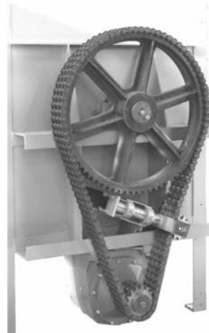
transmission by chain with tensioner
