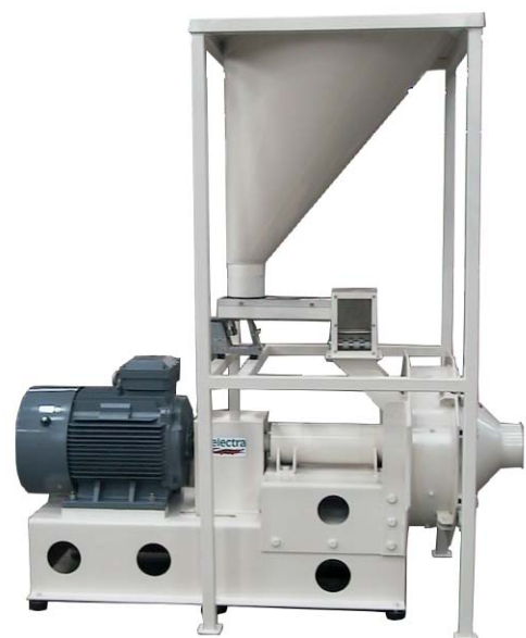
BM 600 with vibrating dispenser
