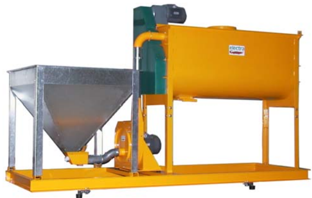
Feed production plant mounted on weighing frame
