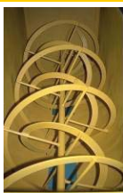
reverse pitch double spiral blades
