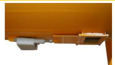
electric actuator to control the slide valve
