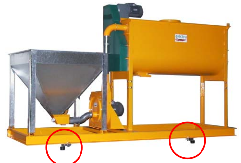
feed production plant mounted on weighing frame
